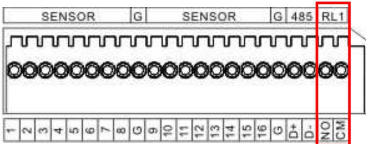
The relay device should be set to NO (Normal Open) and it will change to NC (Normal Close) when an event has been triggered.
