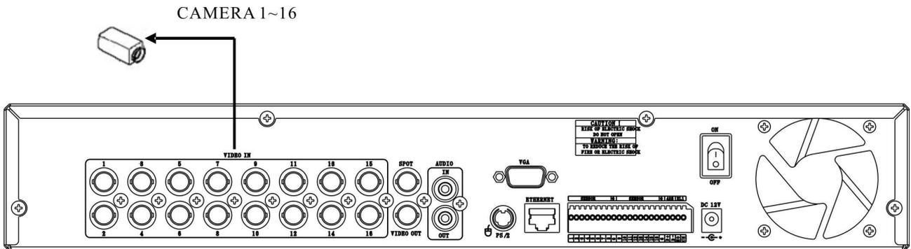
\* Connect a female BNC connector of each camera to a male BNC connector, "CAMERA IN" port.
