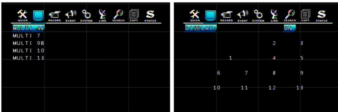
Enter one of the five modes (4, 7, 9 for 8CH and 4, 7, 9, 10, 13 for 16CH) and change the selected channel to multi-split screen. Turn the display on and then it will be shown in the sequence by pressing MULTI or SEQ button on the front panel.
