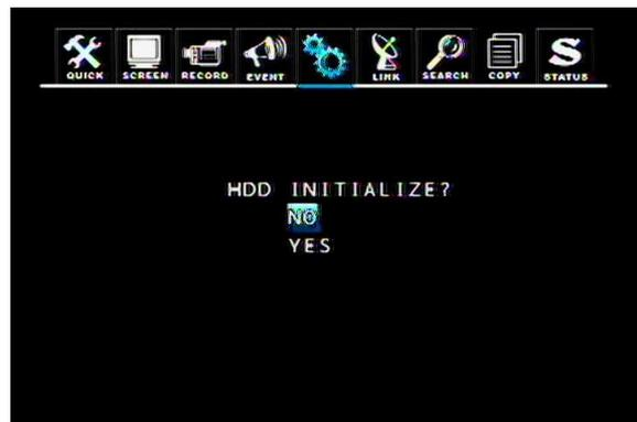
REC HDD INITIALIZE: Select YES and press ENTER button to format the HDD.
