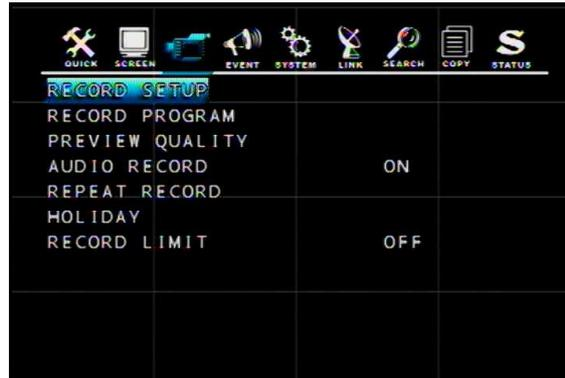
If QUICK SETUP setting is "OFF", DVR will record data according to the RECORD SETUP settings. DVR provides 10 RECORD PROGRAMs, user can use RECORD SETUP menu to arrange the different RECORD PROGRAMs to different time point. For example, you can use higher recording frame to record on workday, and use lower recording frame on weekend. The default RECORD PROGRAM is PROGRAM6.
